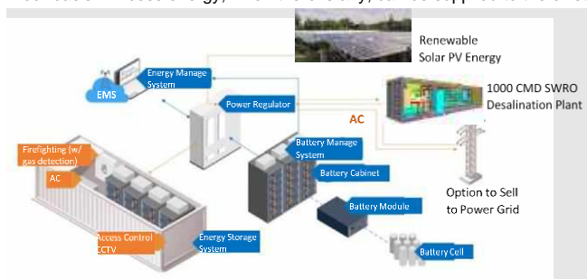
Figure 10. Illustrative diagram of a solar PV energy system attached to the SWRO desalination plant Source: Taboada E.B. et. al., op.cit.
